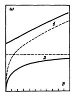
The dashed lines in Fig. 1 show the dependence on the external field  $H_0$  of the frequencies of the electronic (1) (low-frequency branch) and nuclear (2) resonances in the absence of the coupling on the basis of data of [2]. They are of the form
