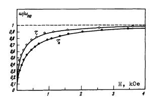
Fig. 2. Dependence of resonant frequency of electron-nuclear resonance on the magnetic field at temperatures T<sub>1</sub> and T<sub>2</sub> of 4.2 and 1.8°K. The solid curves correspond to Eq. (2b).
