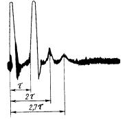
Our experiment was carried out for SbCl<sub>3</sub> (Sb<sup>123</sup>, I = 7/2) and BiCl<sub>3</sub> (Bi<sup>209</sup>, I = 9/2). The sample was placed in a system of two coils, each of which was excited by pulse pairs from separate pulsed hf generators. Since both generators (frequencies  $\omega_1$  and  $\omega_2$ ) were triggered by a single pulse source, both transitions were excited simultaneously by pulses of equal duration.
