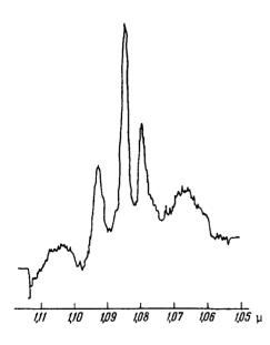
the region near 1000 nm, taken at room temperature with a DFS-12 spectrograph. The center of the most intense line is near 1085 nm, and its width is 2.0  $\pm$  0.1 nm. The lifetime of the corresponding excited state is 85  $\pm$  5 µsec at room temperature. The centers of the two other less intense lines are near 1079 and 1093 nm.
