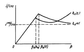
explains the appearance of a drooping section on the current-voltage characteristic when  $\beta > \beta_0$ . When  $\xi_0$  is finite and  $\beta$  large, the current increases. The reason is that, by virtue of the conservation laws, the electrons with  $\epsilon < T\xi_0$  do not interact with the phonons and are acted upon only by the electric field.
