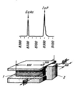
The sample was glued with a dielectric resin to the diode holder. The laser-illuminated strip on the sample was apparently 10-15  $\mu$  wide. The possibility of attaining generation depends in critical fashion on accurately setting the sample in such a way that this illuminated strip is strictly perpendicular to the mirrors.
