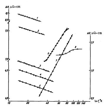
x-ray data, all the samples were single-phase. It turned out that the R-T curves of the iron solutions in alloys with x = 0.01, 0.02, 0.05, 0.1, and 0.2 exhibit a pronounced minimum at  $T = 40^{\circ}$ K. According to our investigations of the magnetic susceptibility, the localized magnetic moment of these alloys remains constant. It can be assumed that in this case the electron-phonon component of the resistance remains unchanged.
