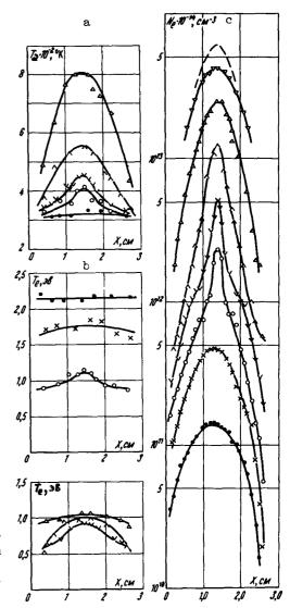
conductivity  $W_T$  and the diffusion energy transfer  $W_D$ . For example, at p = 1 mm Hg and i = 1 A we have at the center of the discharge  $W_D = 4 \times 10^6$  (erg-cm<sup>3</sup>/sec) and  $W_T = 3 \times 10^6$ , while the elastic losses are  $W_{el} = 6 \times 10^5$ . The diffusion flux to the wall exceeded the volume recombination in the charged-particle balance at all the investigated currents (up to 5 A).
