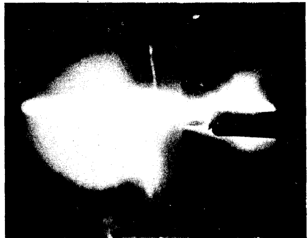
Fig. 1. Photograph of spark in the "slow combustion" mode in the case when the threshold of the effect is exceeded 2.4 times. Linear scale 1:1. Part of the spark image on the right of the photograph is covered. The laser beam moves from left to right.
