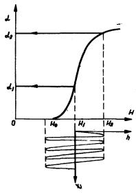
Fig. 2. Magnetization curve of film in a rotating film.  ${\rm H}_{\rm O}$  - threshold value of recording field, determined by the coercive force of the film relative to the domain rotation.
