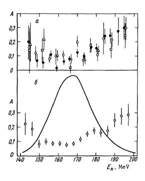
Anisotropy of the  $\gamma$ -quantum yield vs. fragment kinetic energy in the fission of U<sup>235</sup>. a) for different fragmentmass ratios:  $\Box$  -  $m_1/m_2$  = 1.1 - 1.25,  $\Delta$  -  $m_1/m_2$  = 1.25 - 1.35, • -  $m_1/m_2$  = 1.35 - 1.45, • -  $m_1/m_2$  = 1.45 - 1.65,  $\Diamond$  -  $m_1/m_2$  = 1.65 - 1.9; b) for all realized mass ratios. The solid curve shows the fragment kinetic-energy distribution.
