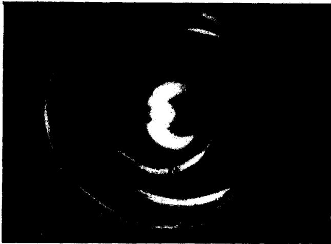
Fig. 1. Pattern of anti-Stokes SRS components in calcite, observed at \nu = 4.02 \times 10^{-2} . The main circles of the first and second anti-Stokes components are seen concentric with the laser spot, and additional circles of the same components are displaced to the right.
