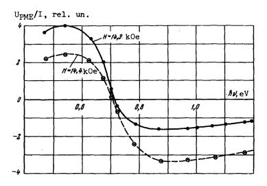
the odd PME in the interval 0.5 - 1.2 eV are shown in the figure for one of the samples and for different values of the magnetic field. Similar curves were obtained for the other samples. It is seen from the figure that at a specified value of the magnetic field the PME voltage reverses sign with increase in frequency and becomes negative, starting with it = 0.7 eV. This quantity agrees with the theoretical value obtained in [1]:
