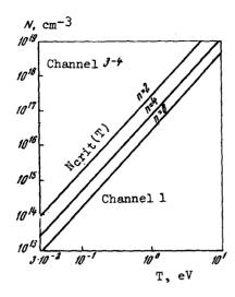
Fig. 2. Regions of predominant decay at the level n of a hydrogenlike ion (Z = 2) through different channels (see Fig. 1).
