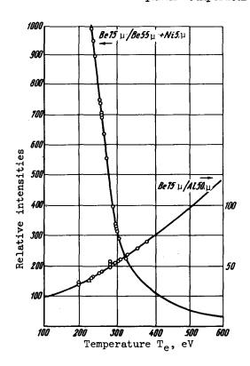
Experimental results of the measurements of the electron temperature  $T_e$  of a laser spark in air and in a mixture of air with deuterium.  $\Box$  -theoretical curves, o - experimental points for air at p=80 mm Hg,  $\Delta$  - experimental points for a mixture of air at 70 mm Hg + deuterium at 100 mm Hg.
