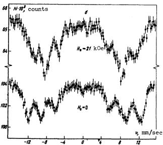
Mossbauer absorption spectra of  $Sn^{119}$  nuclei in  $Gd_{2.7}Ca_{0.3}Fe_{4.7}Sn_{0.3}O_{12}$  iron garnet in a transverse magnetic field and in the absence of a field: a - at  $T = 300^{\circ}K$ , b - at  $T = 95^{\circ}K$ .
