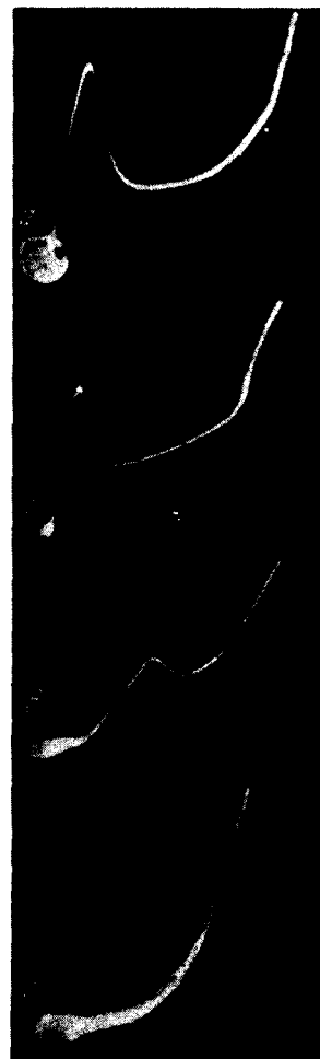
Fig. 3. Current-voltage curve as a function of uniaxial compression along the [111] axis at T = 4.2^\circ\text{K} : P = 0 (a), P = 50 \text{ kg/cm}^2 (b), P = 100 \text{ kg/cm}^2 (c), P = 300 \text{ kg/cm}^2 (d).
