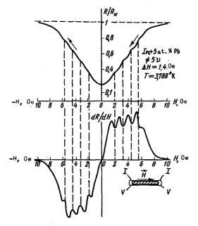
temperatures near critical. The samples were prepared by drawing a glass capillary with the molten metal. The glass was not removed from the sample. The figure shows a typical R(H) plot obtained for a sample of approximately 5  $\mu$  diameter and 4 mm length. The same figure shows a plot of the derivative dR/dH. The amplitude of the field modulation was 0.1 G.
