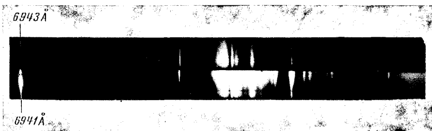
Fig. 2. Spectra of vitrified solution of cryptocyanine in glycerine following a 2 Å change of the exciting wavelength, demonstrating the shift of all the lines.
