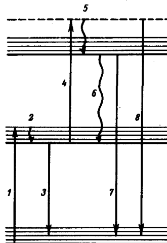
Fig. 1. Energy-level and transition scheme: 1 - absorption of laser quantum, 2 - relaxation to lower states, 3 - single-quantum luminescence, 4 - absorption of laser quantum with transition to virtual level, 5 - relaxation to lower states, 6 - nonradiative relaxation to first excited state, 7 - luminescence from second excited state, 8 - anti-Stokes Raman scattering.
