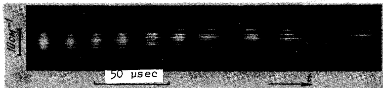
Fig. 3. Scanned spectrum of the neodymium-glass laser spikes.
