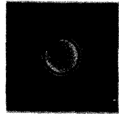
Fig. 3. Image of active surface of a source immersed in liquid argon. Active-region diameter 35 mm, liquid layer 0.4 cm. The bright ring around the active region is due to the reflection of the light of the sparks from the rounded part of the polished electrode (Fig. 1c).
