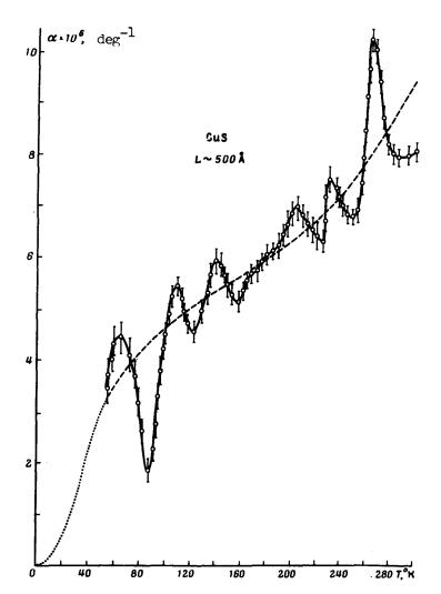
Temperature dependence of the coefficient of linear thermal expansion of semiconducting CuS film 500 Å thick.
