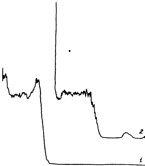
Fig. 3. Distribution of oscillation intensity along the system at 3000 MHz, plotted at different receiver sensitivities. Curve 2 was obtained with a sensitivity 10^3 larger than curve 1.
