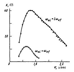
single-crystal yttrium-iron-garnet. The power of the 1.3 GHz signal was  $10^{-10}$  W. A pump of 2.6 GHz frequency and 0.5 W power was turned on at a time  $\tau$  after the application of the signal. The duration of the exciting pulses ranged from 70 to 300 nsec. The enhanced echo pulse was registered at the frequency 1.3 GHz.
