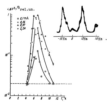
Noise voltage vs. sample temperature for different values of the direct current. The currents 0.1 and 0.36 mA correspond to the linear section of the current-voltage characteristic. The dashed line shows the noise level of the apparatus. The upper right corner shows the form of the oscillogram on the spectrum-analyzer screen.
