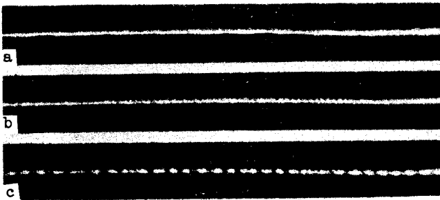
Fig. 2. Oscillograms illustrating different diode operating regimes: a - stationary diode emission, I/I_{thr} = 1.6 ; b - ultrashort spike regime, I/I_{thr} = 2 ; c - regular spike regime, I/I_{thr} = 2.2 . Sweep duration 10 nsec.
