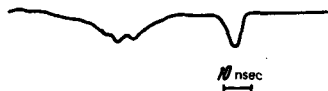
FIG. 1. Oscillogram of the pulses at the entrance (left) and exits (right) of a cell with Rb 2 vapor.
