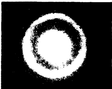
FIG. 1. Distribution of the radiation field of a \text{CdF}_2:\text{Eu} EL cell at a distance 2 cm (cell area 2.5 \text{ cm}^2 ).
