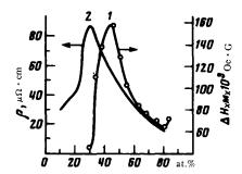
residual resistivity. The figure shows, in accordance with the data of  $^{151}$ , a plot of  $\Delta HM$  against the composition of the FeNi alloy (curve 1). This plot is quite similar to the concentration dependence of the total resistivity of these alloys at 0°C (curve  $2^{161}$ ). If we recognize that with decreasing temperature the peak of the resistivity shifts towards larger Ni concentrations, then the similarity of the two curves becomes even more striking.
