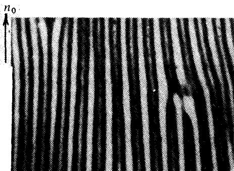
FIG. 2. Modulated structure at T < T_0 in sample (b): n_0 \uparrow —direction of initial orientation, layer thickness 35 \mu , external electric field perpendicular to the plane of the layer.
