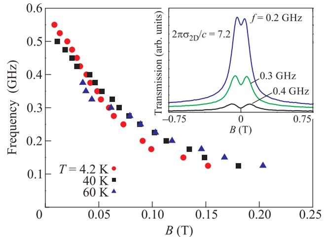
Fig. 2. (Color online) Magnetodispersion of the lower branch in a sample with  $w = 50 \mu\text{m}$ ,  $t = 40 \mu\text{m}$  and an electron density of  $1.8 \cdot 10^{11} \text{ cm}^{-2}$  measured at different temperatures. Inset shows  $B$ -field dependencies of the microwave transmission measured for several microwave frequencies at  $T = 4.2 \text{ K}$
