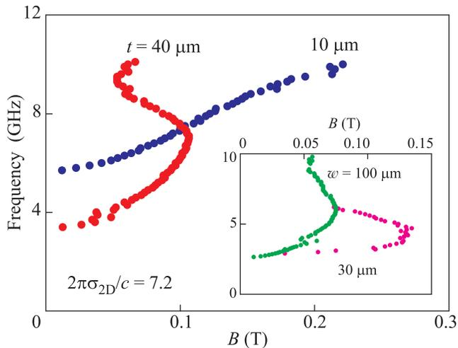
Fig. 4. (Color online) Magnetic field dependencies of the plasma mode for samples with equal 2DES widths  $w = 50 \mu\text{m}$  and different gate widths:  $t = 10$  and  $40 \mu\text{m}$ . The inset shows the Magnetic field dependencies of plasma mode for samples with equal gate widths  $t = 40 \mu\text{m}$  and different 2DES widths:  $w = 30$  and  $100$
