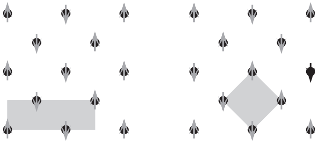
Fig. 1. FeSe AFM configurations studied in the present work: Double-stripe configuration with propagation vector (\pi, 0) (left) and single-stripe configuration with \mathbf{Q} = (\pi, \pi) (right). Shaded areas show the magnetic unit cells
