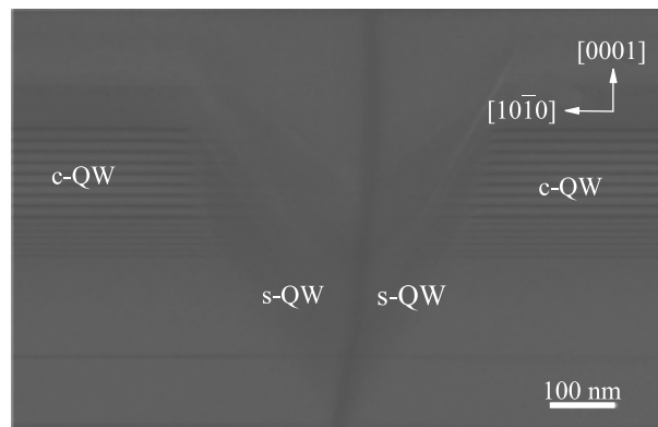
Fig. 1. Dark-field HRTEM images of V-defects in the InGaN/InGaN MQW
