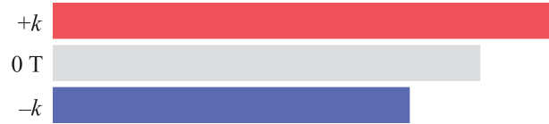
Fig. S2. Transition probability diagram in relative units. The transition from the ground to the nearest excited spin level of the \text{Fe}^{2+} ions is considered
