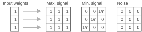
Fig. S3. Weight matrices for calculation of the maximum possible array scale.
